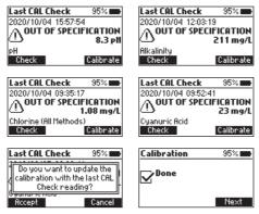
"OUT OF SPECIFICATION": A user calibration is not allowed, the measured value is outside of the
