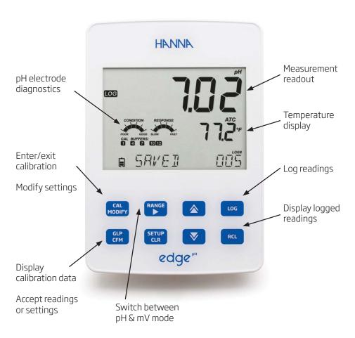
**Flexibility:** A hybrid meter gives you the option to use it as a benchtop instrument or carry it to where you are measuring. A built-in battery will give the greatest versatility.
