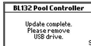
9. Wait until countdown (bottom right corner) reaches 0. Remove the USB drive. The device enters measurement screen.
